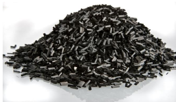
Chopped Carbon Fiber: Tenax®-E HT C604 6mm
