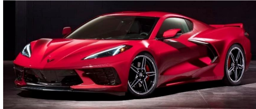
GM Chevrolet Corvette Body panels for doors, fenders, etc. (Glass fiber composites)
