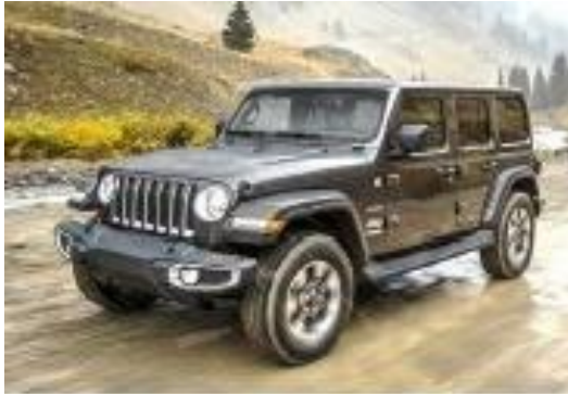
Jeep Wrangler Roof Freedom Panels (Glass fiber composites)
