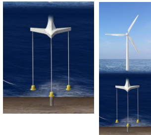
Aramid: Mooring ropes for offshore wind power generation
