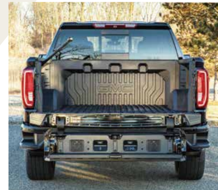
General Motors' pickup truck for which the Sereebo CFRTP is used as a material for the pickup box
